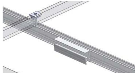
By using the Clenergy splice kit you don't need to cut the rails.
